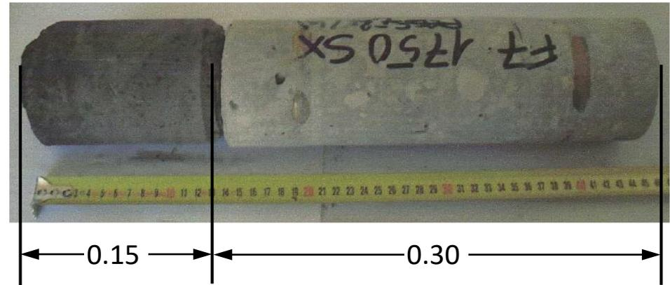
$$\left. \begin{aligned} \bar{K}_{grout} &= 2.5 \cdot 10^{-10} \text{ m/s} \\ \bar{K}_{concr} &\cong 10^{-11} \text{ m/s} \end{aligned} \right\} \bar{K}_{lining} = 1.5 \cdot 10^{-11} \text{ m/s}$$
