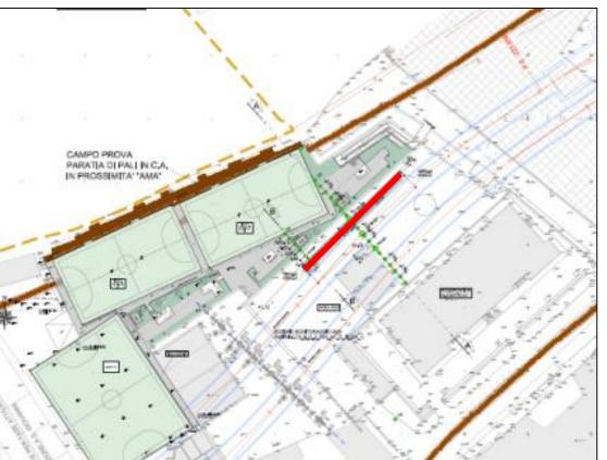
installation to be completed by January 2016 48 concrete piles D = 600 mm; L = 34.5 m spacing = 900 mm (=1.5 D) instrumentation:
