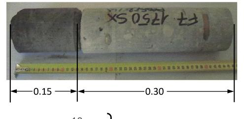
$$\overline{K}_{\text{grout}} = 2.5 \cdot 10^{-10} \text{ m/s}$$
