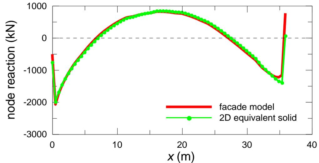
node reactions to given displacements
