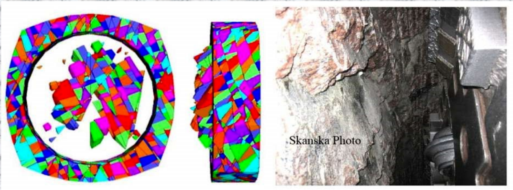
3DEC model of block instability due to low in situ stresses
