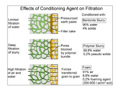
This concentration of air in the crown area reduces the support pressure in that sensible area and consequently causes overexcavation. The air diffusion, on the other hand, stiffens the muck and facilitates its transportation and deposition.
