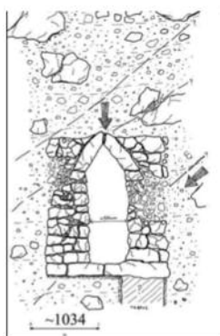
Figure 10. Tunnel in colluvium. Damage of the archaic lining (ch. 1034).
