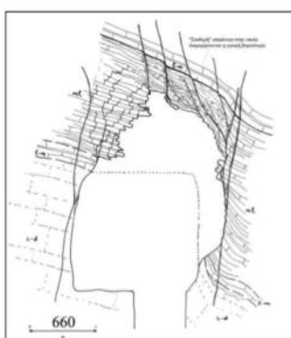
Figure 12. Instability on the roof in thin-bedded horizons (ch. 660).
