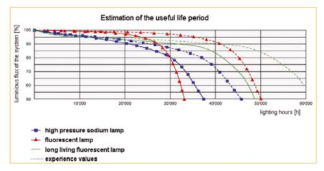
FIGURE 18 - COMPARISON OF LIFE PERIODS OF TYPICAL TUNNEL LAMPS
