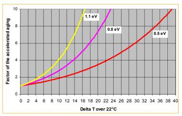
FIGURE 14 – ACCELERATED AGEING AS A FUNCTION OF THE DIFFERENCE BETWEEN ACTUAL OPERATION TEMPERATURE AND 22 DEGREES. THE DIFFERENT ACTIVATION ENERGIES REPRESENT DIFFERENT MATERIALS.
