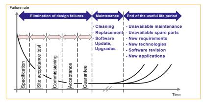
FIGURE 20 - ADAPTED BATHTUB CURVE FOR TECHNICAL EQUIPMENT INCORPORATING SOFTWARE
