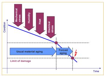
FIGURE 16 - DIFFERENT STRESSES SHOWN FOR ENERGY CABLE
