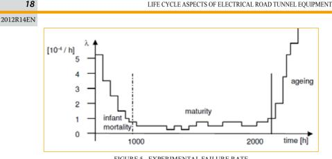
FIGURE 5 - EXPERIMENTAL FAILURE RATE
