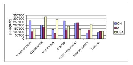
FIGURE 11 – AVERAGE REPLACEMENT COSTS PER ANNUM FOR 3 TYPICAL TUNNELS BASED ON – AVERAGE LIFE CYCLES COLLECTED IN THE SURVEY
