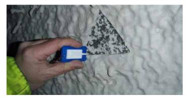
Figure 8: Optional method with cut-out inspection patches to establish the applied membrane thickness
