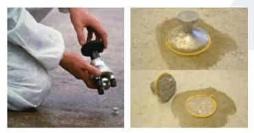
Figure 9: Tensile bond test of horizontal substrate with elcometer. Dolly before and after testing (on the right)
