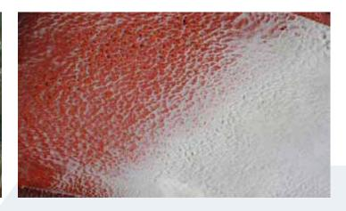
The two layers of membrane were in contrasting colours: the first in orange, the second in white/grey. This approach allowed the thickness of the membrane to be controlled and allowed for easier quality control checking of the application.
