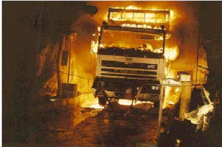
Figure 3: Fire test on a heavy good vehicle loaded with 2 t of modern furniture
