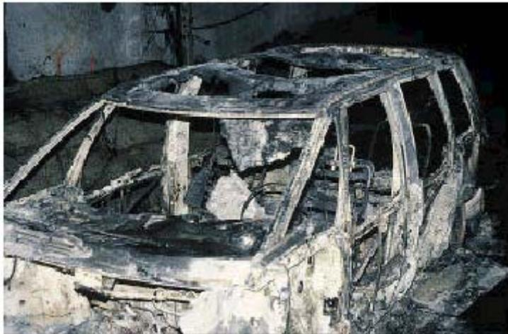
Figure 2: Plastic car Renault Espace completely burnt down in a fire test within the EUREKA project EU 499.
