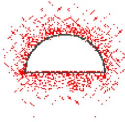
Figure 9: Extent of failure zone surrounding the tunnel top heading in a rock mass defined by GSI = 45. Shear failure is represented by the · symbol while tensile failure is denoted by the ○ symbol.
