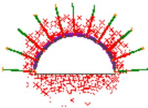
Figure 10: Reduced failure zone in the top heading roof due to the installation of untensioned fully-grouted rockbolts and steel fibre reinforced shotcrete.
