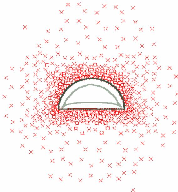
Figure 11: Failure zone surrounding the tunnel top heading in the Daj Khad shear zone, defined by a Geological Strength Index of 20. The tunnel convergence, shown by the deformed excavation boundary, is approximately 400 mm.
