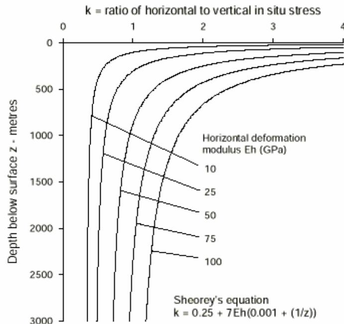
Figure 2: Ratio of horizontal to vertical in situ stress versus depth below surface. (Sheorey 1994)
