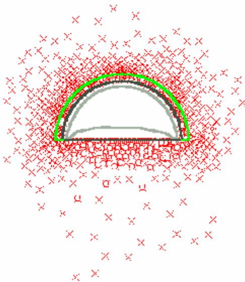
Figure 12 : Failure zone surrounding the forepole umbrella used to support the tunnel top heading in the Daj Khad shear zone. The size of the failure zone and the magnitude of the roof displacements, compared to those shown in Figure 11, have been significantly reduced.
