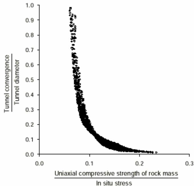
Figure 8: Convergence of an unsupported tunnel versus ratio of uniaxial compressive strength of the rock mass to in situ stress.
